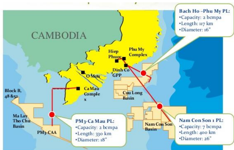
PICTURE OF CURRENT GAS PIPELINE OF VIETNAM
